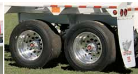
Super single tires with aluminum wheels
