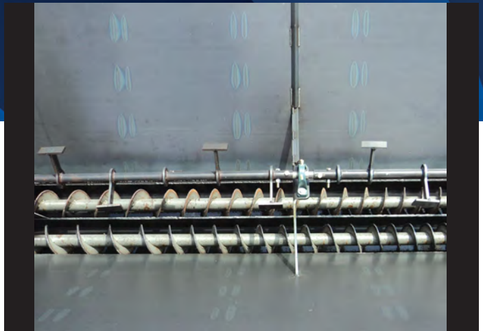
Duel Conveyor System For standard or large rapid asphalt repair and eliminates asphalt bridging.
