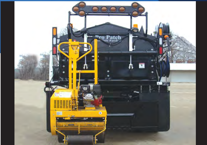
Dump body (4 or 5 cubic yards) LP or CNG gas heating system. 80 or 120 Emulsion tank. Class 50, 40 ton hoist tack spray and hydraulic tools.
