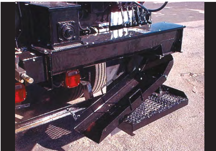
Asphalt Edger Designed to repair deteriorated shoulders on highways and long trenches.
