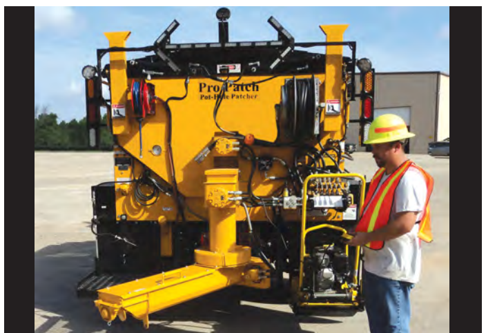
Swing Auger Used to repair large cut and long trenches. Available in manual or remote control.
